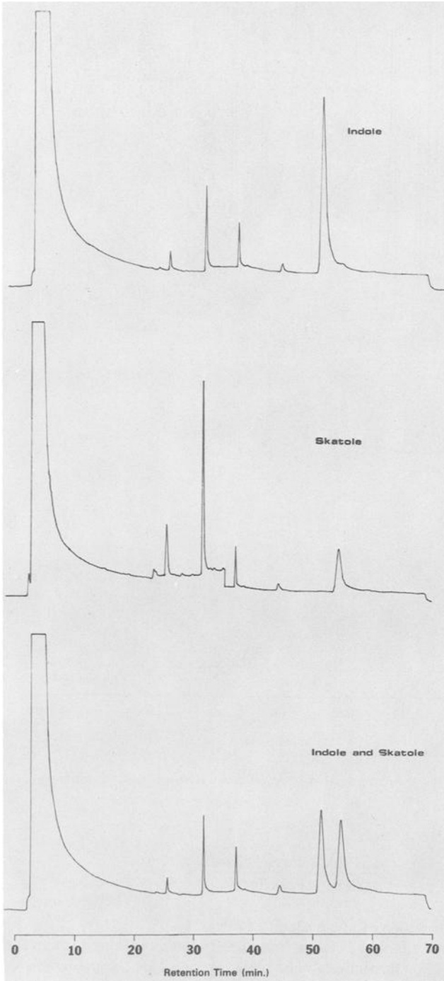
FIG. 5—Chromatograms of 1 mg/100 mL solutions of indole, skatole, and indole plus skatole.
